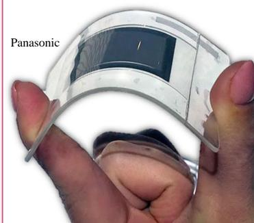
**Panasonic** – A flexible battery that can pass 1000 bend cycles and maintain 80% of the capacity. At 0.45 mm, it is very thin, but with a low max capacity of 60 mAh, much less than an iPhone 7 battery (~1900 mAh). (2017)
