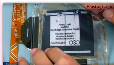
**Cambridge Graphene Centre and Plastic Logic** – Flexible e-ink type display using graphene electronics. (2014)
